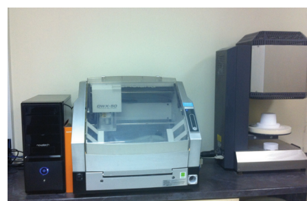
Figure 2: Roland 5 axis in-house milling machine and sintering furnace
