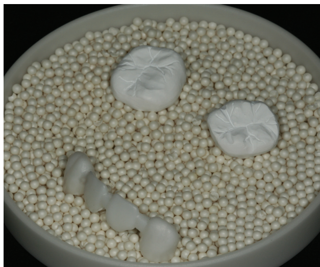
Figure 3: Zirconia full contour and framework bridge ready for sintering
